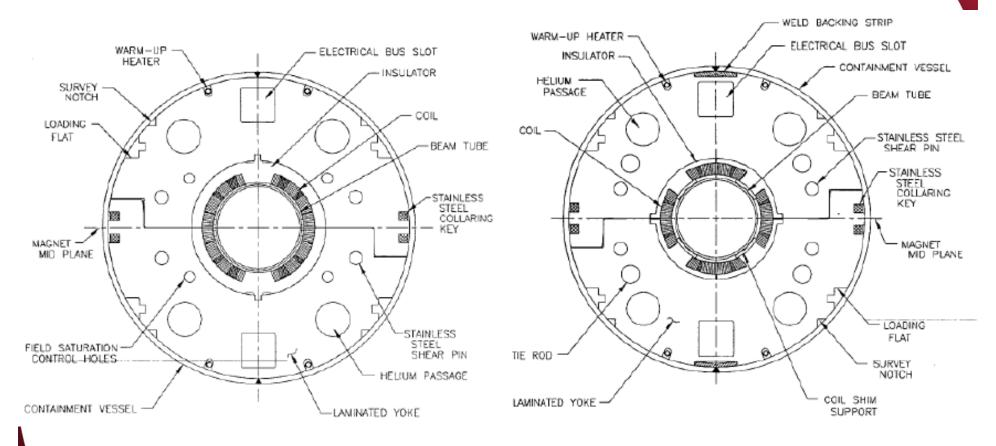
RHIC cos(θ)-style superconducting magnets and yokes NbTi in Cu stabilizer, iron yokes, saturation holes Full field design strength is up to 20 Mpa (3 kpsi)
