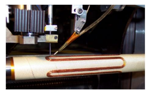
World's first "direct wind" coil machine at BNL
