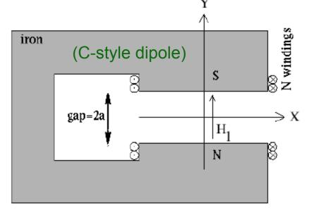
Field integral is through N-S poles and (highly permeable) iron (including return path)
