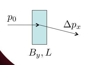
$$F_x = \frac{\Delta p_x}{\Delta t} = q(\beta c)B_y \quad \Delta t = L/(\beta c)$$
