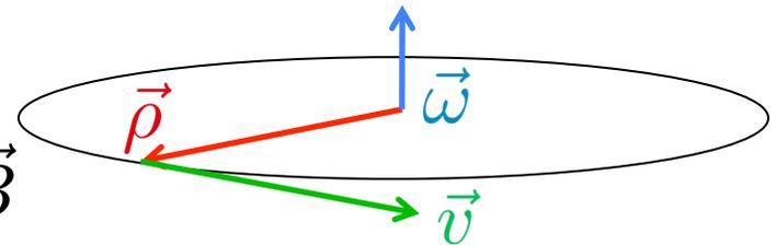
$$\vec{v} = \vec{\omega} \times \vec{\rho} \quad \Rightarrow \quad q\vec{v} \times \vec{B} = \gamma m \vec{\omega} \times \frac{d\vec{\rho}}{dt} = \gamma m \vec{\omega} \times \vec{v}$$
