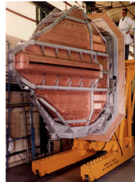
Fig. 26: Outer shell of resonator, with support frame and beam slit
