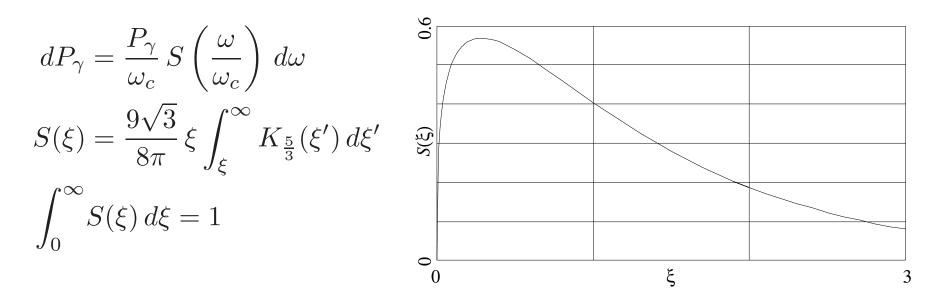
• Critical energy: half the power is radiated by photons less than the critical energy, and the other half, above.
