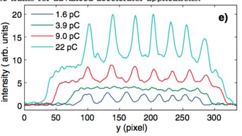
Space-charge driven plasma oscillations modify initial modulation from SCRF gun
