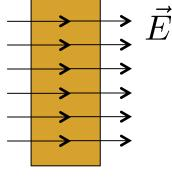
normal to surface points out of paper  $\theta = 90^{\circ}$  between  $\vec{E}$  and normal
