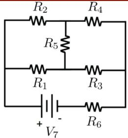
The circuit shown above has resistors  $R_1 = 1.0 \Omega$ ,  $R_2 = 2.0 \Omega$ ,  $R_3 = 3.0 \Omega$ ,  $R_4 = 4.0 \Omega$ ,  $R_5 = 5.0 \Omega$ , and  $R_6 = 6.0 \Omega$  connected by perfectly conducting wires. The EMF  $V_7$  has a voltage across its terminals of  $V_7 = 12.0 \text{ V}$ . This circuit cannot be reduced to just parallel and series capacitors; you have to use Kirchhoff's rules to evaluate it.
