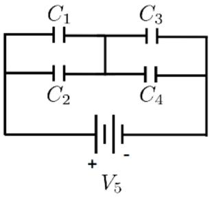
The circuit shown above has capacitors  $C_1 = 1.0 \ \mu\text{F}$ ,  $C_2 = 2.0 \ \mu\text{F}$ ,  $C_3 = 3.0 \ \mu\text{F}$ , and  $C_4 = 4.0 \ \mu\text{F}$  connected by perfectly conducting wires. The EMF  $V_5$  has a voltage across its terminals of  $V_5 = 12.0 \text{ V}$ , and the circuit is in a state where the capacitors are charged.
