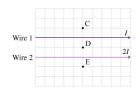
2. Consider the wires in the above figure, with the top wire carrying current I to the right and the bottom wire carrying current 2I to the right. In what direction is the *total* magnetic field from these two wires...
