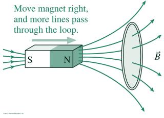
Moving a magnet near a wire loop increases the flux through the loop. The result is an induced EMF given by Faraday's law. The induced EMF drives an induced current in the loop.
