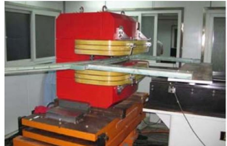
PEFP prototype magnet (Korea) 9 cm gap, 1.4m long
