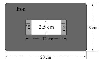
(a) (4 points) Estimate the number of ampere-turns necessary to achieve a 0.6 T field in the gap. Assume that the iron is not saturated, so the relative permeability is roughly  $\mu_r \equiv (\mu/\mu_0) = 5000$ .
