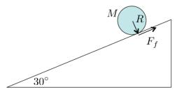
A uniform sphere of radius R and mass M is placed at the top of a plane inclined at an angle of  $\theta$ . The coefficient of friction between the plane and the ball is  $\mu$ . Gravity acts vertically downward as in most inclined plane problems.
