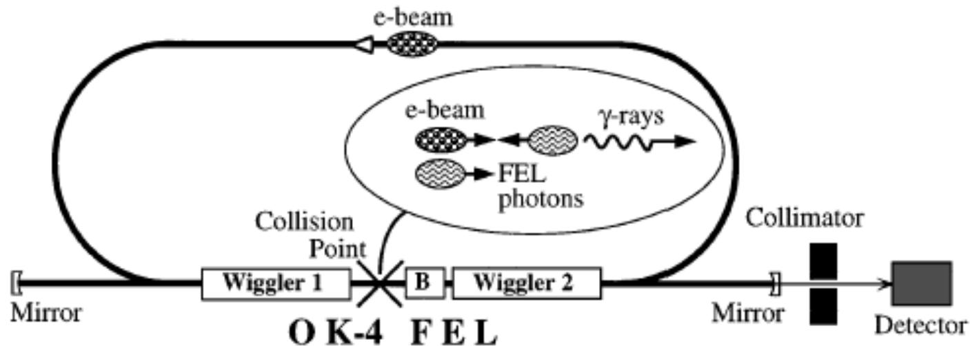
FIG. 1. Schematic of the OK-4/Duke storage ring FEL and  $\gamma$ -ray source. Two electron bunches spatially separated by one-half the circumference of the ring participate both in lasing and  $\gamma$ -ray production via Compton scattering of intracavity photons. A collimator installed downstream selects a narrow cone of quasimonoenergetic  $\gamma$  rays.
