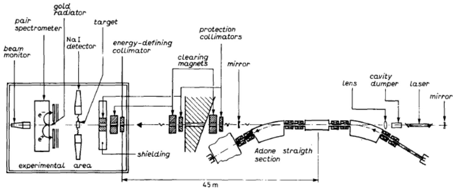
Fig. 1. – Overall view of the experimental set-up.
