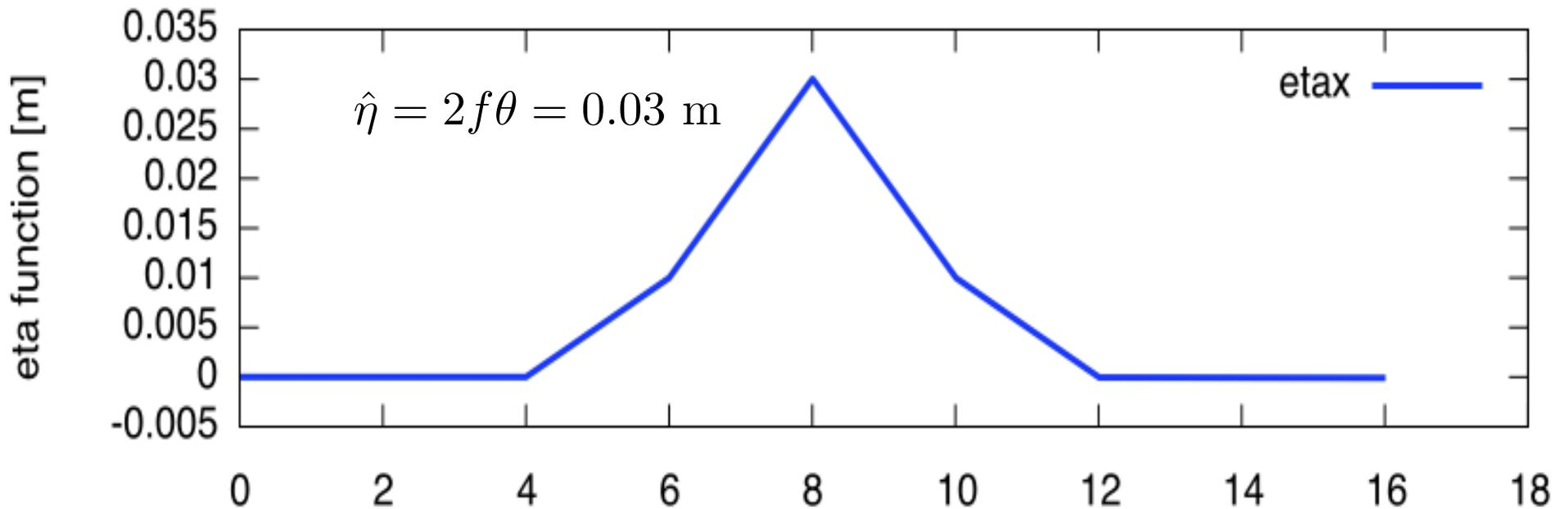
$$L = l = 2 \text{ m} \quad \theta = 0.01 \text{ rad} \quad f = \frac{L + 2l}{4} = 1.5 \text{ m} \quad (KL_{\text{quad}}) = 0.667 \text{ m}^{-1}$$
