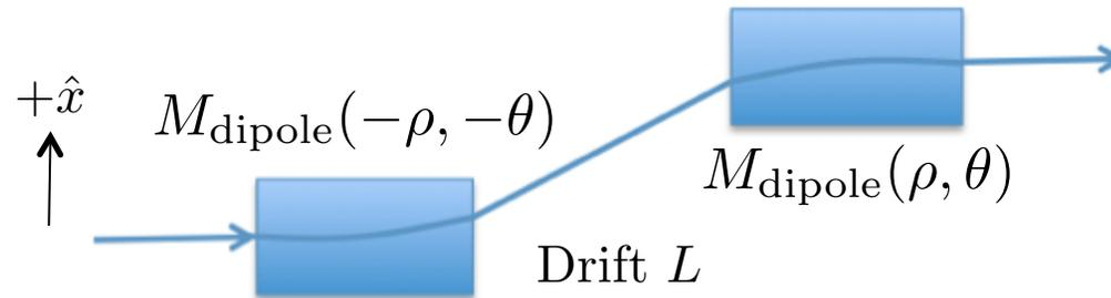
$$\mathbf{M}_{\text{dogleg}} = \mathbf{M}_{\text{dipole}}(\rho, \theta) \mathbf{M}_{\text{drift}} \mathbf{M}_{\text{dipole}}(-\rho, -\theta)$$
