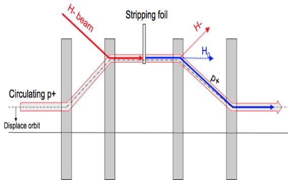
Figure 2: Visual representation of the charge-exchange injection for the JLEIC  $H^-$  ion beam leaving the linac and being stripped of its electrons to create a proton beam in the Booster synchrotron
