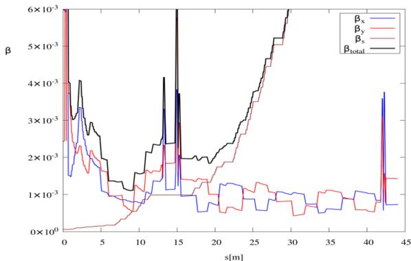
Figure 7: RMS relativistic velocities along the JLEIC ion linac
