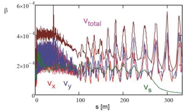
Figure 6: RMS relativistic velocities along the SNS linac [4]
