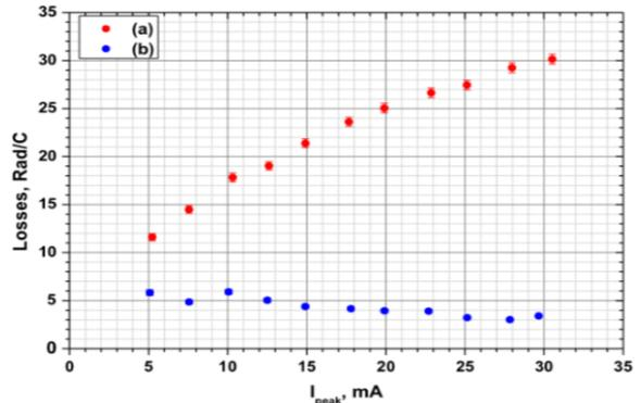
Figure 3: The beam loss in the SNS linac vs peak current for (a)  $H^-$  ions and (b) protons [2]
