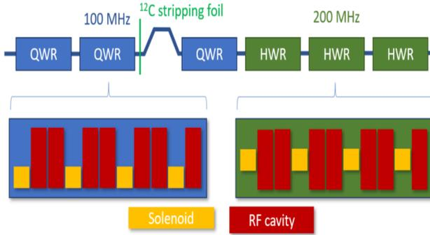
Figure 4: Diagram of the ordering of the JLEIC superconducting ion linac elements
