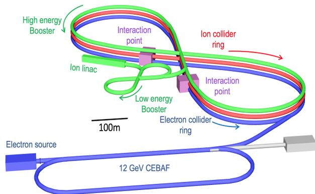
Figure 1: JLEIC facility design with the superconducting linac located between the Ion Source and Booster synchrotron
